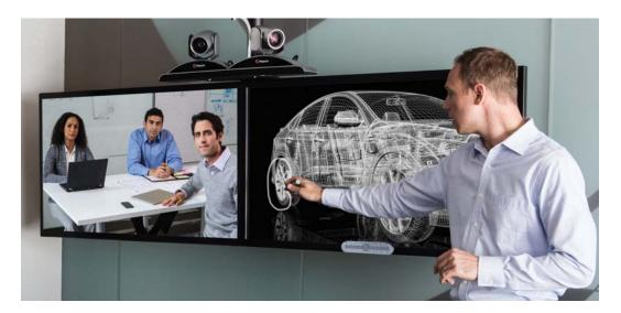
Two monitors are required to use the Polycom UC Board. The second monitor can be either a projector used with a whiteboard, or a monitor.
