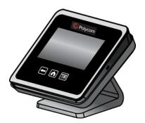
Users can connect to one another using a shared address book, on-screen keypad, and calendar entry. For quick access to room information, the Polycom Touch Control communicates with the RealPresence Group
