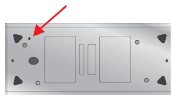
The restore button pinhole is on the front of the Polycom RealPresence Group 700 system, as shown in the following figure.
