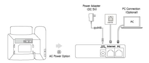
**Note** The IP phone should be used with Yealink original power adapter (5V/600mA) only. The use of the third-party power adapter may cause the damage to the phone.
