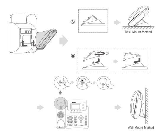
**Note** The hookswitch tab has a lip which allows the handset to stay on-hook when the IP phone is mounted vertically.
