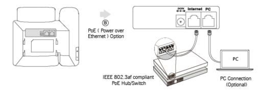
**Note** If in-line power is provided, you don't need to connect the phone to the power adapter. Make sure the switch/hub is PoE-compliant.
